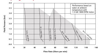
E2P10-XXXXX-AX-XXA Maximum Outlet Working Pressure 100 PSIG (6.89 bar). End user piping design must be rated to withstand this pressure.
