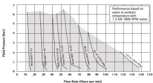
E2P10-XXXXX-CX-XXA Maximum Outlet Working Pressure 190 PSIG (13.1 bar). End user piping design must be rated to withstand this pressure.
