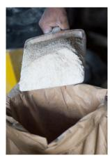
There are several powder transfer methods, each with its own unique benefits and challenges. The most basic of these methods is the manual charging of powders into downstream processing equipment. Manual handling is slow and can delay production as well as present countless opportunities for messy spills and cross-contamination
